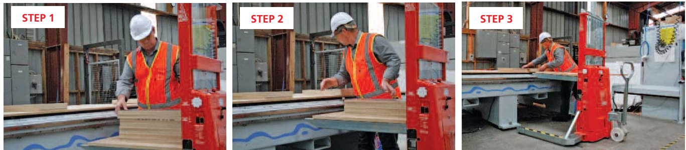
Unloading timber onto conveyor using auto infra-red eye sensor
