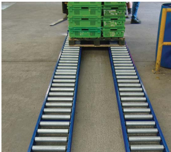
Pallet conveyor mounted to the warehouse floor to transport pallets from the packing line to the pallet wrapping area
